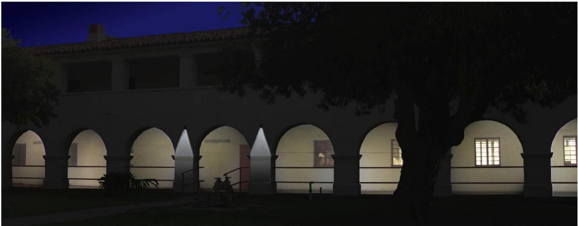
Note that the actual light sources are concealed and provide uniform illumination to minimize glare while the illuminated surfaces create a soft and comfortable visual environment. Building entrances are illuminated with downlighting for wayfinding.
