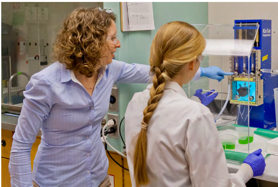
Christal Sohl (San Diego State University) trains graduate student Anna Uvarova (now employed at Novartis in Boston) to use a rapid quench to measure how quickly polymerases replicate DNA.
