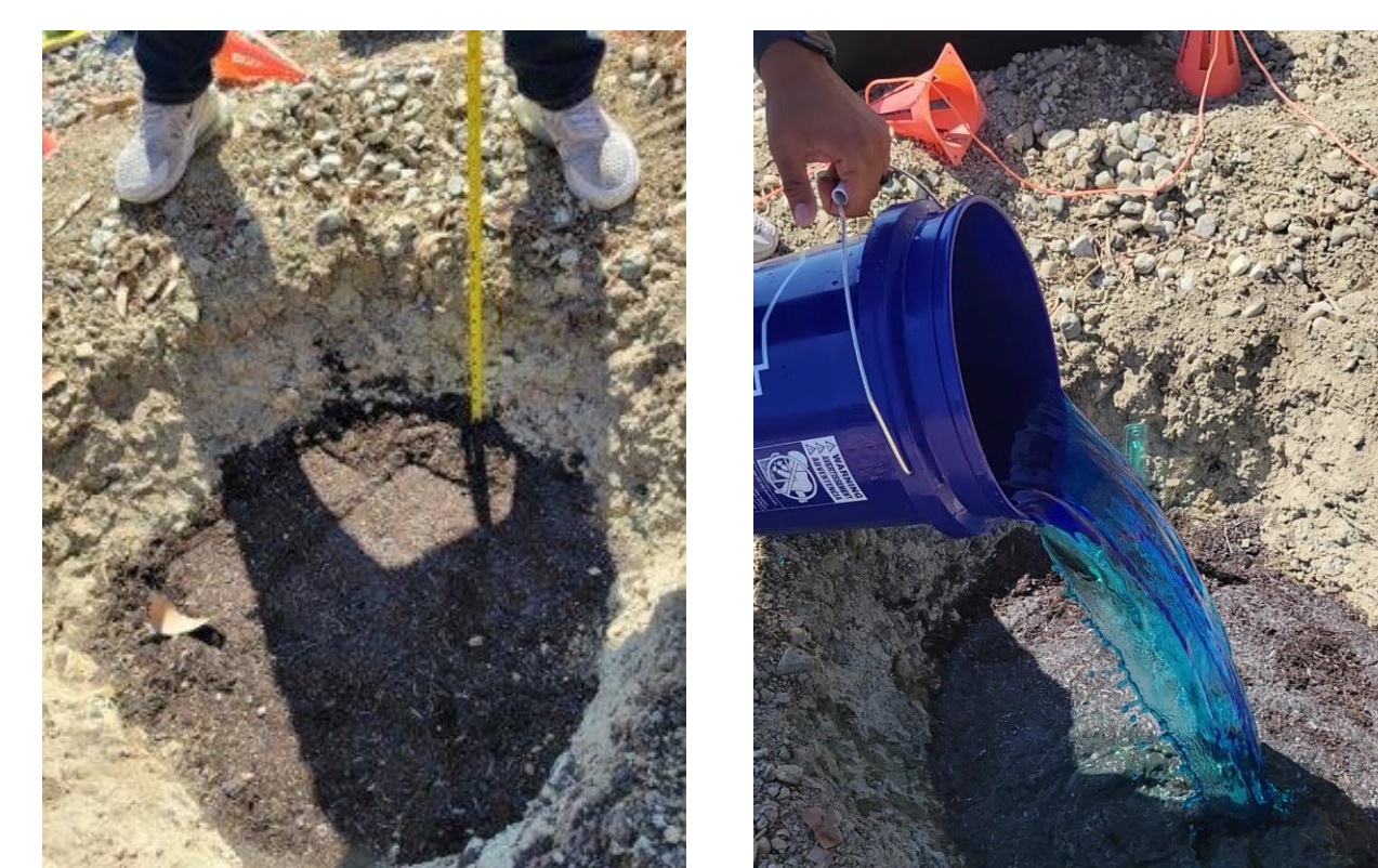
Percolation test with manure added
