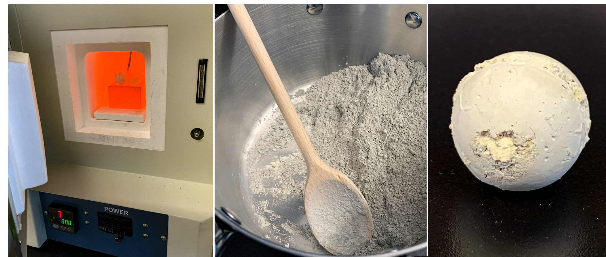
Heating of Calcium carbonate to form Calcium Hydroxide (Lime)
